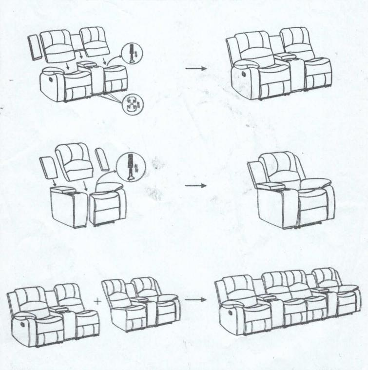
**CONSOLE CAN BE EXCHANGED LEFT AND RIGHT**
